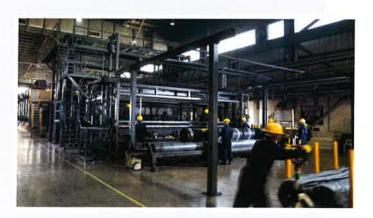
Coating - The greige fabric obtained from the processes described above is taken onto a one-of-a-kind, ultramodern coating machine where it is coated with a proprietary SBR based coating compound, which lends it durability, dimensional stability, and resistance to installation damage.
