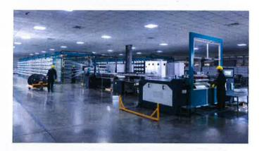
Beaming - A predetermined number of yarn ends are pulled from a creel and wound onto a large cylindrical beam. The beaming machines are fully automated which ensures uniformity in yarn tension, take up and unwinding stability.
