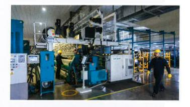
Knitting - High tenacity polyester yarn is precision knitted into a dimensionally stable network of apertures that serves as a highly stable, high modulus precursor to the coating process.
