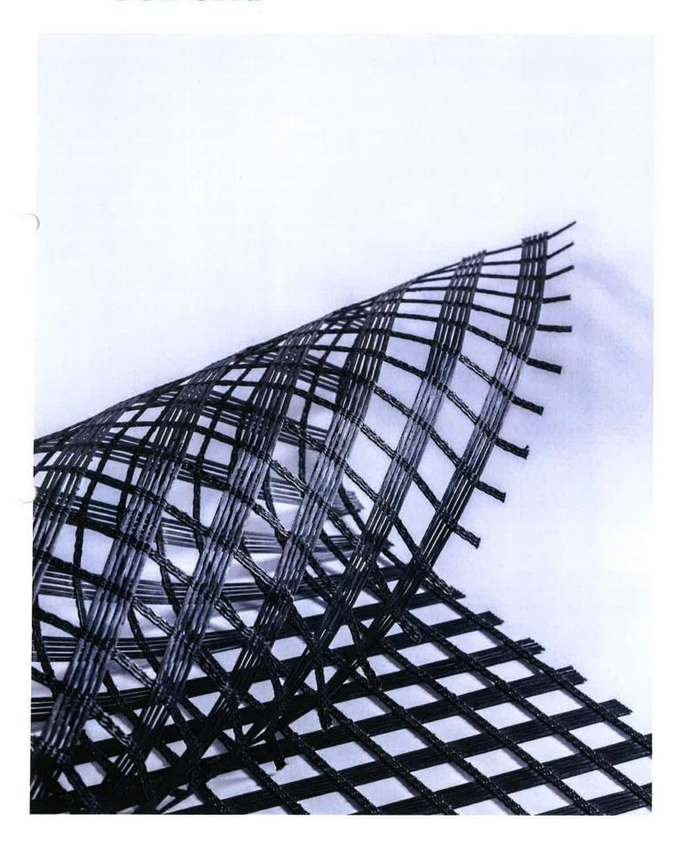
StrataGrid™ Biaxial (SGB Grid) is a high-performance reinforcement geogrid, engineered specifically for improving the modulus values of the pavement base layers. The SGB Grid series has undergone substantial testing for performance and quality control. It is manufactured with high tenacity polyester yarns with industry-leading stress-strain values to provide the highest tensile resistance at lower elongations.
